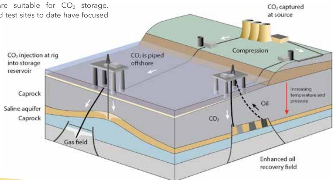
Right: schematic cartoon showing the principles of offshore carbon capture and storage, including the use of CO<sub>2</sub> injection in Enhanced Oil Recovery (EOR). After AFP, European Commission, USGS.
