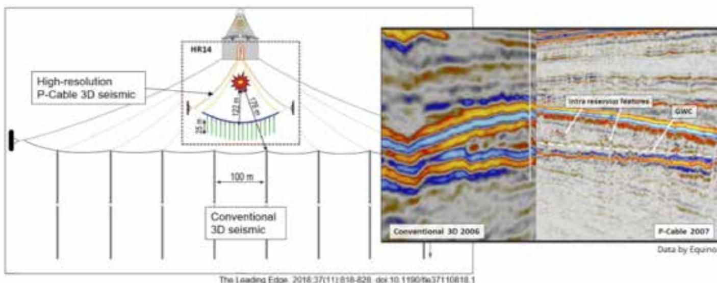
Above: Comparison of high-resolution P-Cable and conventional 3D seismic system layout and data resolution.
