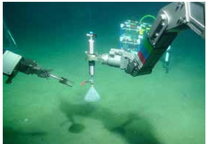
Top: Deployment of the CO<sub>2</sub> gas containers from the back of the RRS *James Cook*. Middle: An anxious wait - Doug awaits the first sighting of bubble at the seafloor. Bottom: Sampling the escaped gas with the ROV.
