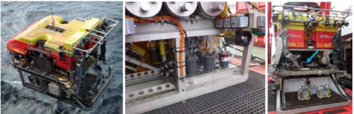
Figure 2 - Left: ISIS being deployed with the LOC sensors just visible in the bottom left of the vehicle. Middle: Rear view of ISIS, showing the LOC sensors mounted on the rear starboard bottom corner on their aluminium sled. Right: Front view of ISIS with the position of the intake pump marked with a blue arrow.
