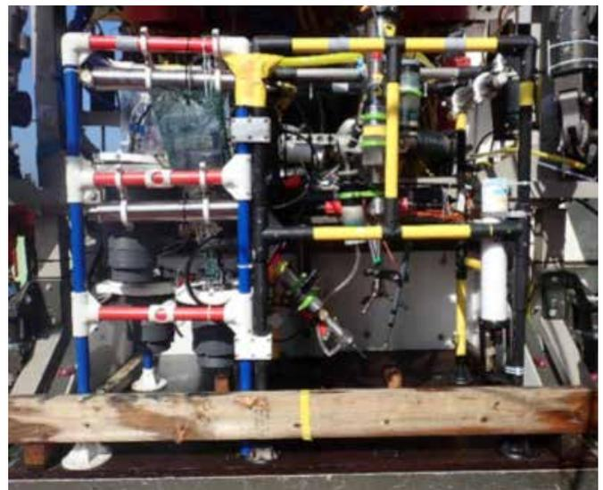
Figure 1. A benthic boundary layer lander on the tool sled of the ROV immediately before deployment. Eddy covariance instruments are mounted on the right. Lab on chip sensors are mounted on the left.
