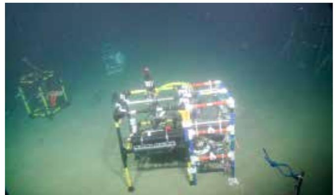
Figure 3. The MPI BBL lander on the busy seafloor around the bubble emission zone. The right half of the lander (with the blue and red frame) contains five LOC sensors with their associated reagents, standards, and batteries.
