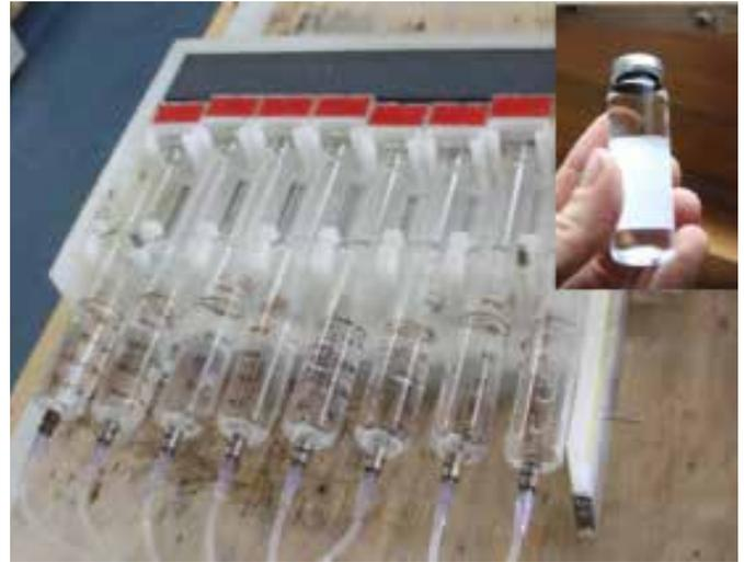
Above: Syringes filled with samples of the water within the benthic chambers that were collected at regular intervals throughout the incubation. These samples were carefully stored in gas-tight vials (inset) that will be analysed at on-shore laboratories in UK and Germany.
